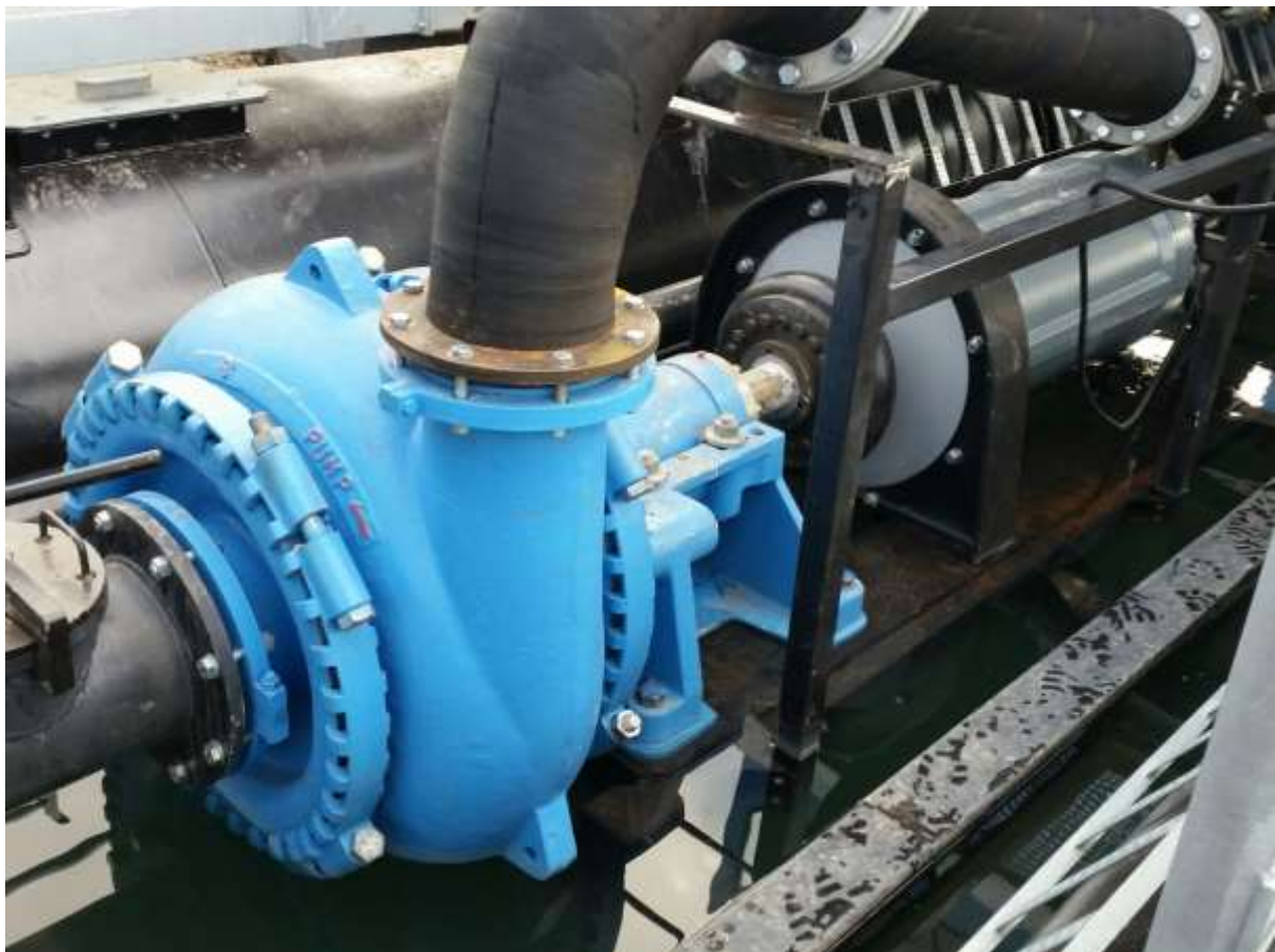
Picture 10: SPG 10/8 FU-G with DTZ underwater seal
