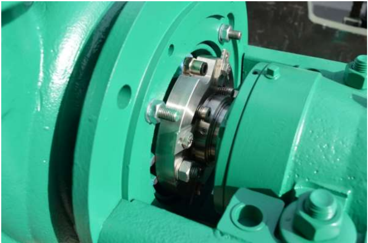
Picture 9: DTZ mechanical seal mounted in SPG 3/2 pump
